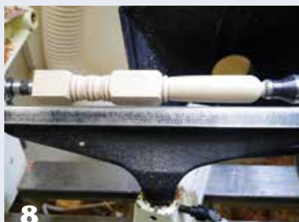
8 The spokes are first turned between centers, then mounted in a chuck to gain access to the handle ends.
