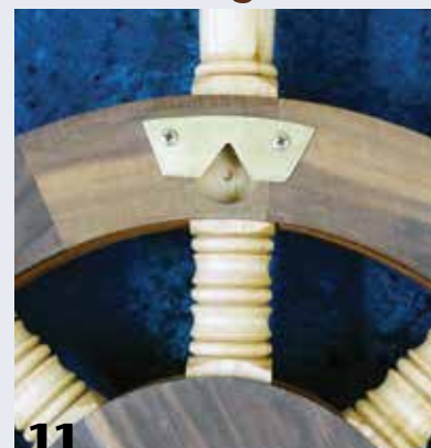
11 A rear-facing hole and notched brass plate serve as a worthy hanger.
